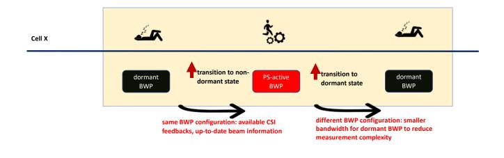
FIG. 3 Dormant SCell Mechanism
