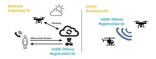
FIG. 4 Two types of Remote Identification (RID)
